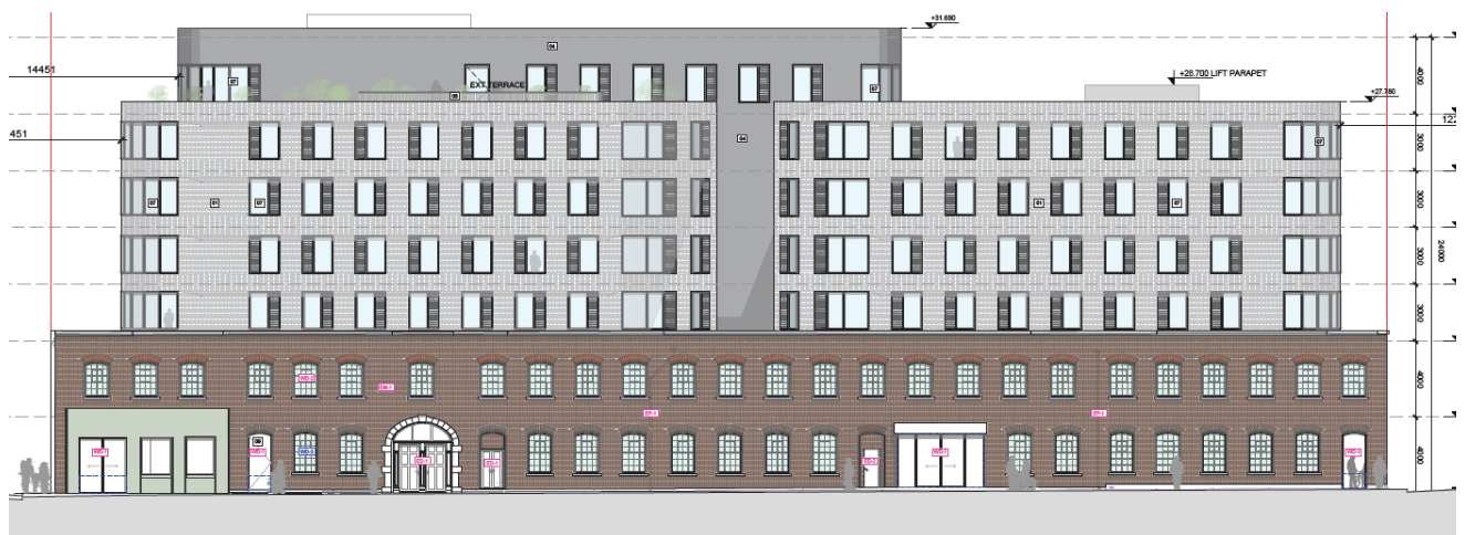
Fig. 23 Proposed elevation of retained north façade onto North King Street, with proposed new building behind (reproduced from Architectural Design Report by MOLA)
